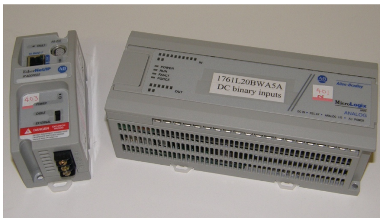
Figure 7-15. The Allen-Bradley MicroLogix 1000 PLC. The PLC, the unit on the right, has analog and binary I/O ports. Its communications is handled by the 1761-NET-ENI unit shown on the left, p. 7-17
