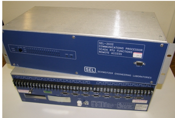
Figure 19: Modern SCADA unit. This is the SEL-2032 (front view on top, back view on the bottom). 115
