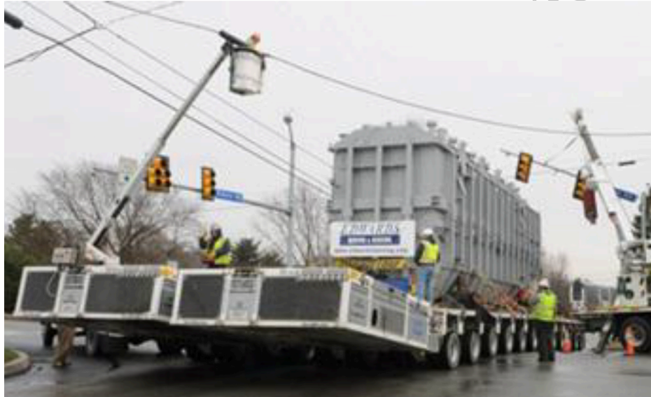
Figure 6: Workers move wires, lights, and poles to transport a 340-ton LPT, causing hours of traffic delay. LPTs can weigh up to 400 tons, four times more than rail transport can handle. 52
