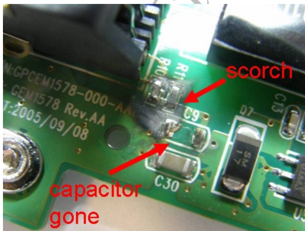
Figure 6-2. Capacitor damage from pulse testing. The capacitor (C9) is gone, and there are scorch marks (C30 shows an undamaged capacitor), p. 6-2
