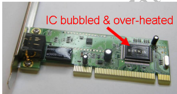
Figure 18: Integrated circuit (IC) damaged by large electrical pulse. The IC lid, normally flat, has bubbled, and is discolored from overheating. 113
